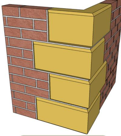
Leg and height dimensions usually coincide with brick sizes For Example: typical leg lengths 465mm & 240mm and typical height 215mm or 290mm
