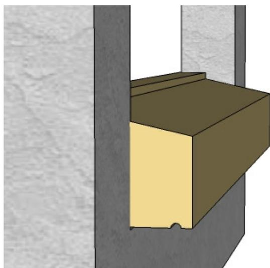
Slip cills can sit flush with the window opening or extend along the front edge of the wall
