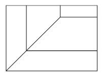
Beam End Built Into Wall 100mm Minimum
