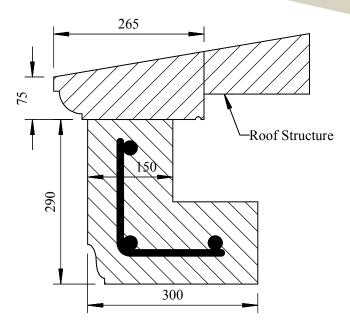
Roof structure not supplied; to be arranged by customer
