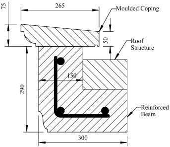
Roof structure not supplied; to be arranged by customer
