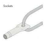
Example of a lifting socket we would cast into a stone
