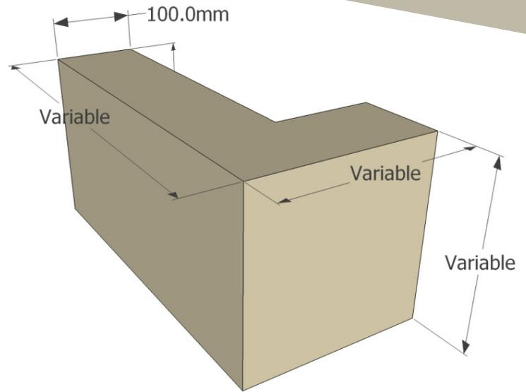
Standard return quoins are built into the wall, forming part of the structure. - see our cladding quoins if you intend to fix the stones after the wall is built.
